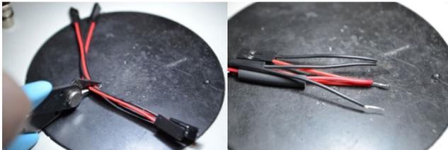
Using the two female halves and the leftover male end from the yellow LED strip, strip approximately 1/2" of the insulation on the end of all of the wires. Place a 1" piece of small diameter shrink tube over the red wire and another on the black wires of one piece. Solder the red wires together, push the shrink tube over the joint and shrink it with a heat gun till it's tight on the joint.
