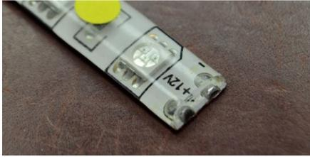
Using a Xacto knife carefully peel away the waterproof coating. This is easier if you first cut through the coating, but do not cut the strip below the coating. Peel off the coating to reveal the solder connections.
