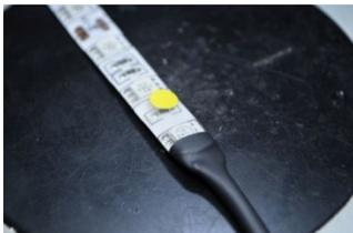
Repeat this process with the red/green and yellow LED strips. Make sure that the red LED strip has a male connector and the green and the yellow LED strip has a female connector. Save the extra cut off male end for later.
