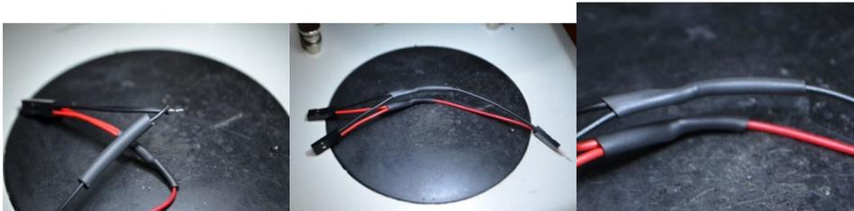
Solder the black wires together and seal the joint with heat shrink. You should now have a connector with one male end and two female ends. Repeat this process to make the second connector. You have enough male ends in the kit to make both connectors.
